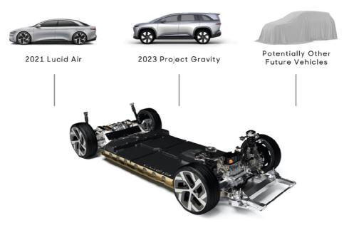
• *Integrated Electric Motor, Inverter and Transmission Drive Unit.* Lucid's motor and gearbox system utilizes permanent magnet motors that were developed in-house. Combining these motors with an inverter and an integrated gearbox and differential creates an advanced 900V+ electric drive unit that weighs just 163lb (74kg) and is small enough to fit inside a carry-on roller bag.
