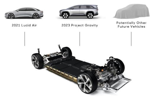
• *Integrated Electric Motor, Inverter and Transmission Drive Unit.* Lucid's motor and gearbox system utilizes permanent magnet motors that were developed in-house. Combining these motors with an inverter and an integrated gearbox and differential creates an advanced 900V+ electric drive unit that weighs just 163lb (74kg) and is small enough to fit inside a carry-on roller bag.
