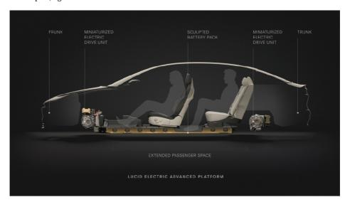
The Space Concept was achieved through a ground-up rethink in the way an automobile is designed. The launch edition of the Lucid Air is expected to have a "bench" style rear seat that provides expansive
